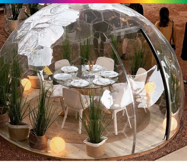
FANUS DOME is a crystal clear dome that blends perfectly with the surroundings. The pocket you're not a maker of transparent hexagonal solid polycarbonate plates with 4 mm stainless screws made of material used in phones.
